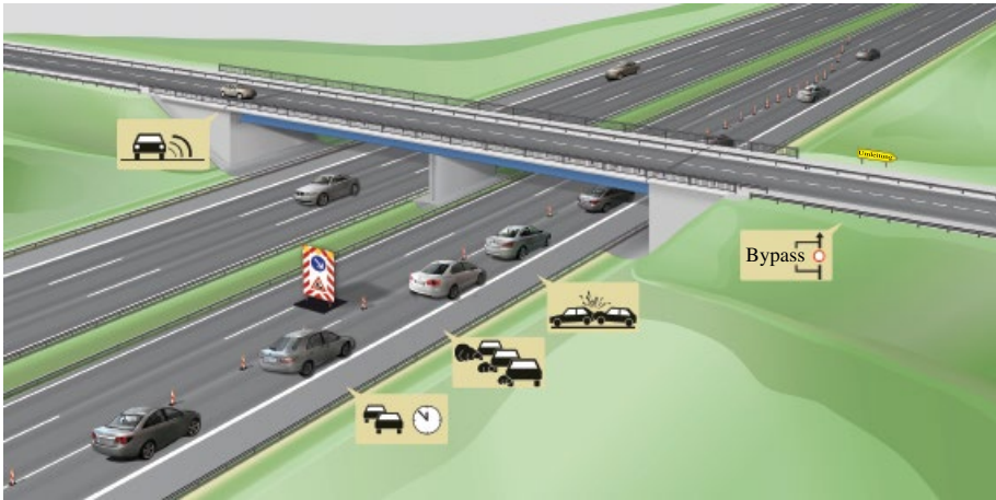
Figure 4.93 External effects important for the assessment of bridges: time delays of users, additional exhaust emissions, changed accident rates and accident likelihood, necessary detours and noise emissions, for example, generated by transition joints.
