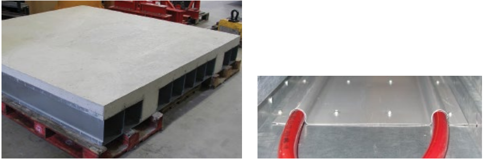
Figure 4.82 Left: test specimen, composite double layer floor. Right: \Omega -profile used to contain the pipes.
