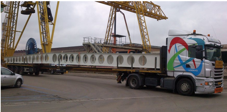
Figure 6.71 Transportation of several cellular beams – delivery length 29.8 m. © ArcelorMittal.
