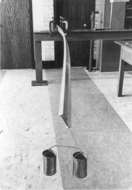
Figure 6.1 Lateral buckling of a cantilever.
